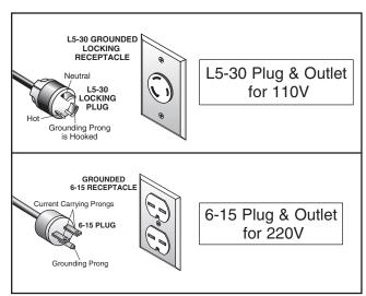
Figure 7. Recommended plug types.
